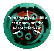
Note, the Adapter's locking mechanism is designed to be used in heavy duty vehicles such as highway trucks and construction equipment and can be very tight to lock. To ease locking and unlocking your Adapter, you can trim away the lower half of the three nipples located on the inside of the ring (see picture above). Be careful that you don't trim too much of the nipples otherwise the Adapter will not lock, in which case you will need to replace the locking ring.
